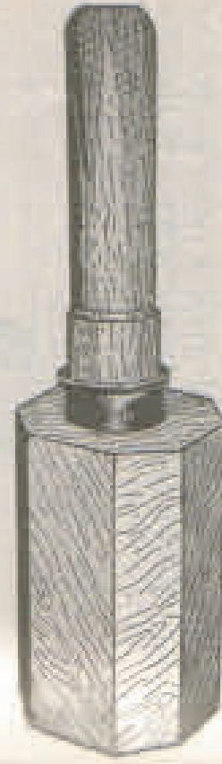
(b) Method of employing hardwood punch and die in straightening nose (ogive).
